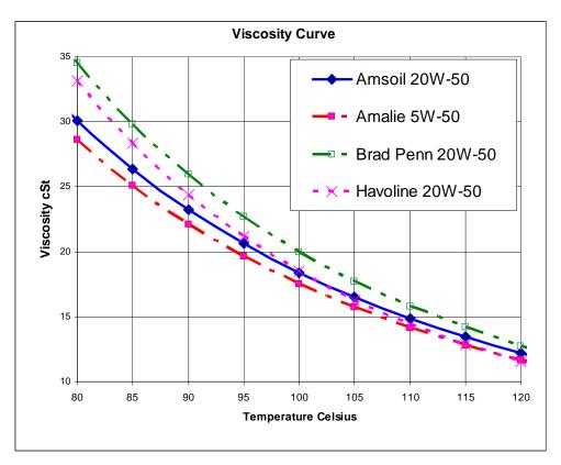
Between 100° C and 105° C the Havoline (and other similar mineral oils) goes from the thickest to the thinnest. Brad Penn maintains the most viscosity, while Amsoil becomes the second most viscous. At about 165° C (temperatures found in turbos) the Amsoil product becomes the thickest.
